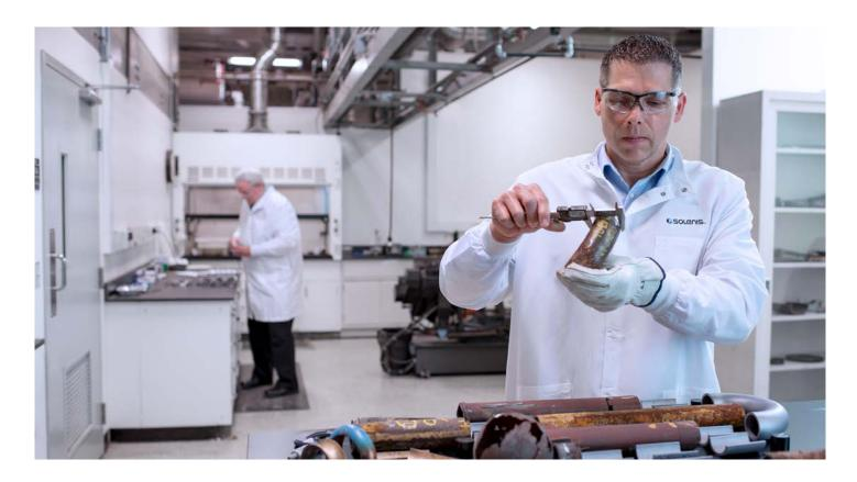
house microbiological, water and deposit analysis laboratories enables a rapid and complete profile of microbiologically influenced corrosion failures.
