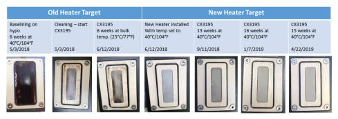
**Reduced Manganese Deposition on Probe**
