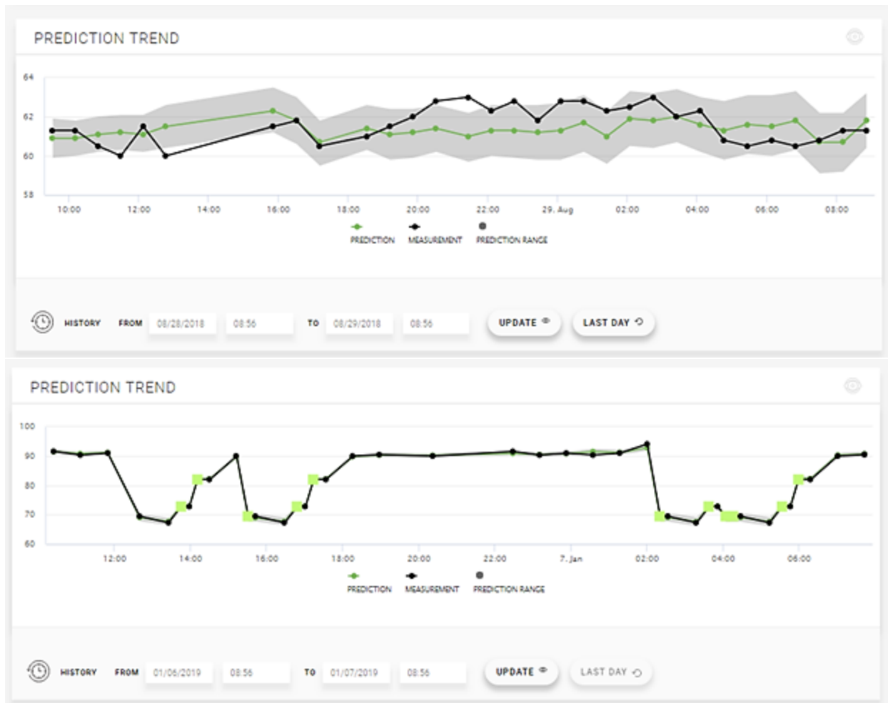
Figure 14. Effect of machine learning on prediction accuracy using papermaking process data: (a) Early stages of simulation; (b) Late stages of simulation resulting in near-perfect predictions
