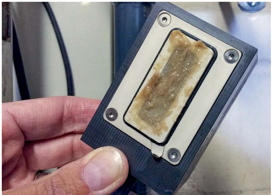
Heated target assembly showing the presence of biofilm
