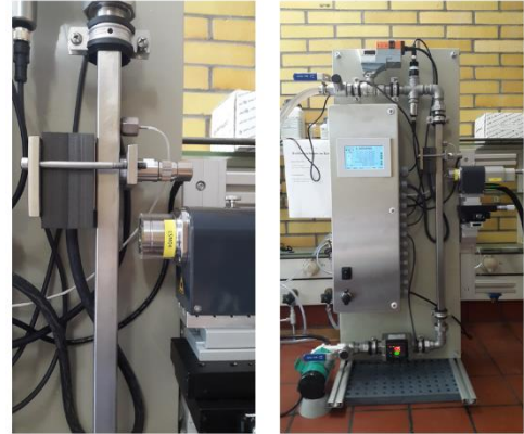
Figure 1: Laboratory set up of the OnGuard 3B analyzer and the OCT camera.
