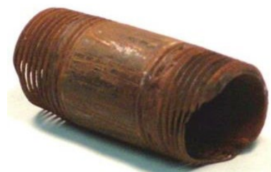
Condensate System Pipe Nipple Thinned By Carbon Acid Corrosion
